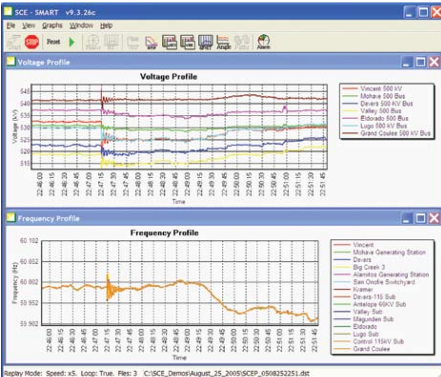
Screen capture of the strip charts produced by Synchronized Measurement and Analysis in Real Time (SMART), SCE's real-time operations tool for phasor visualization.
